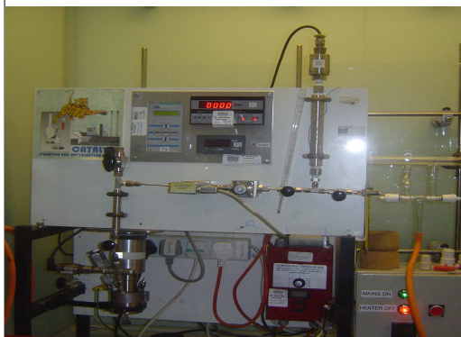
Figure 2: (left) Homogeneous batch reactor setup capable of efficient gas/liquid mixing and the ability for kinetic measurements at constant pressure and volume. Figure 3: (right) Screen shot of Igor showing a: the imported data (in table one) b: data being manipulated (text box, bottom left) c: data presented in graphs (graphs 3 and 0) and d: two examples of data being fitted to mathematical models; graph 3 shows and exponential fit and graph 0 shows a linear fit.
